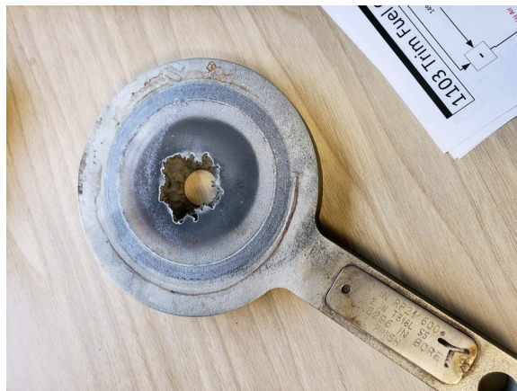
The opposite face: violent destruction at the bore from cavitation collapse.
