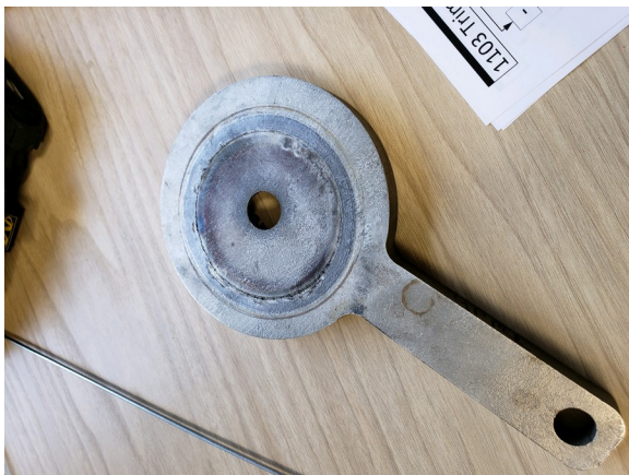
One face: continuous wear across the surface. The bore is still mostly defined.
